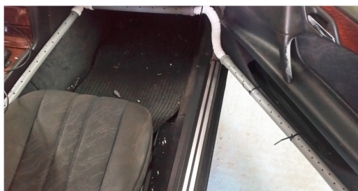
Fig. 3 – The turbulent circular air jets curtain tube-work mounted at the level of the seat
