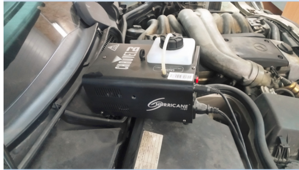
Fig. 4 – Hurricane 1101 smoke generator positioned at the ventilation and air conditioning system intake.
