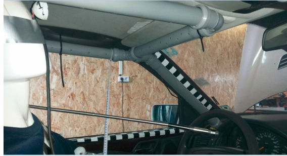
Fig. 19 – Anemometer positioned at the turbulent circular jets curtain at 0.4 m.
