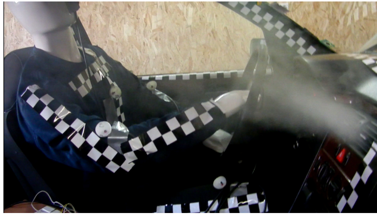
Fig. 6 – Air conditioning jet of the classic system.
